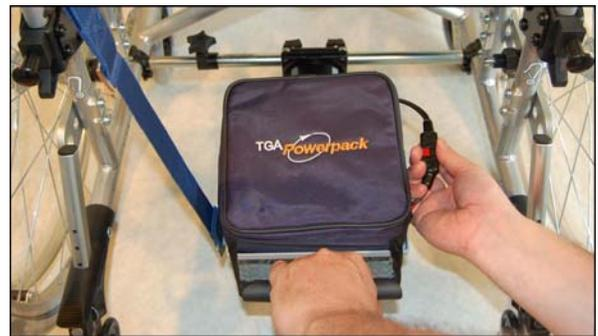
**Fig 7 Fitting and Connecting Battery**
