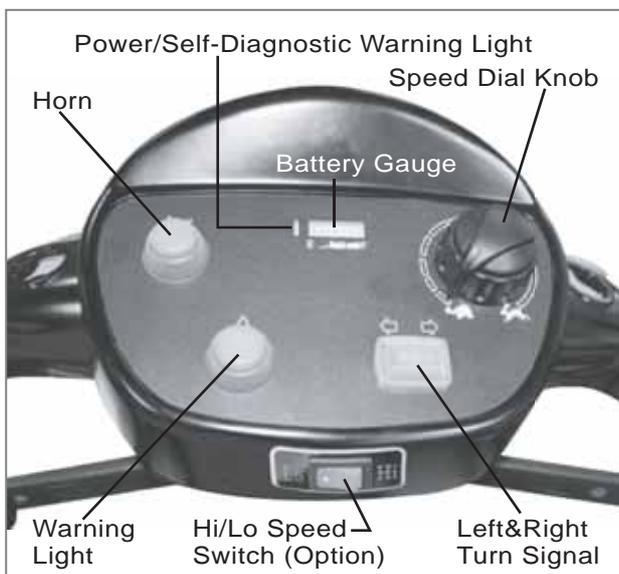
Figure 2 - ST-4E / ST-4D Control Panel
