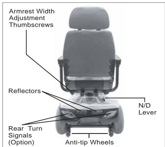
Figure 3 - ST-4E / ST-4D Rear View
