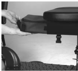
Push/pull battery pack into the battery bracket
