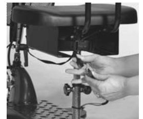
Push the power connectors together
