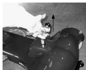
Removing seat lock bracket
