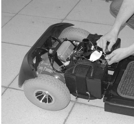
2. Disconnect the batteries by disconnecting the two red connectors and two black connectors.
