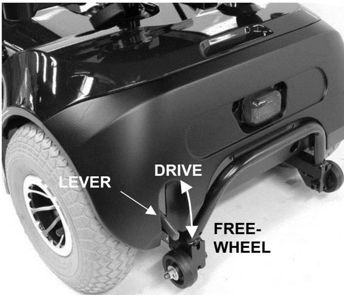
The motor on the scooter can be disengaged to allow the scooter to be pushed .
