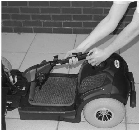
5. Loosen the tiller adjustment knob and fold down the tiller and retighten knob.
