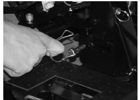
6. Remove the lock pin located to the rear of the seat post and between the batteries.
