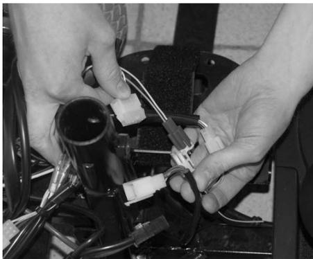
7. Unplug the front-to-rear harnesses. On the Neo 8 only, remove the 'R' clip and pin attaching the rear cable brake.
