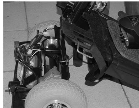
9. Lift the front section until the lower pegs are no longer in the curved locking brackets. Carefully lift the front section away from the rear section.
