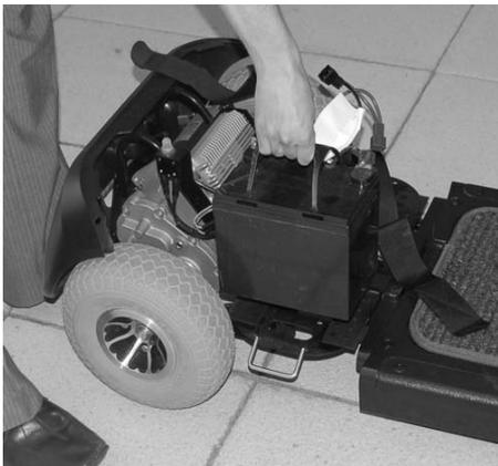
4. Remove the batteries.
