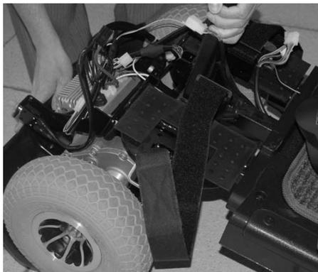
8. Pivot the scooter's rear section upwards until the rear section is standing vertically on its rear bumper.
