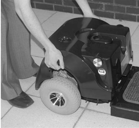
1. Switch off the scooter, unscrew the seat hand wheel and remove seat. Be careful not to let the seat post drop when removing. Lift up the rear shroud to remove.
